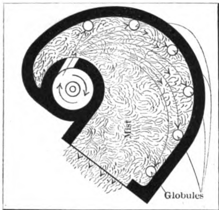
Fig. 5—Section of a snail-like curve offered to illustrate the principle of the vortex
